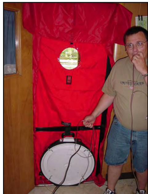
Setting up the blower door for a depressurization test
