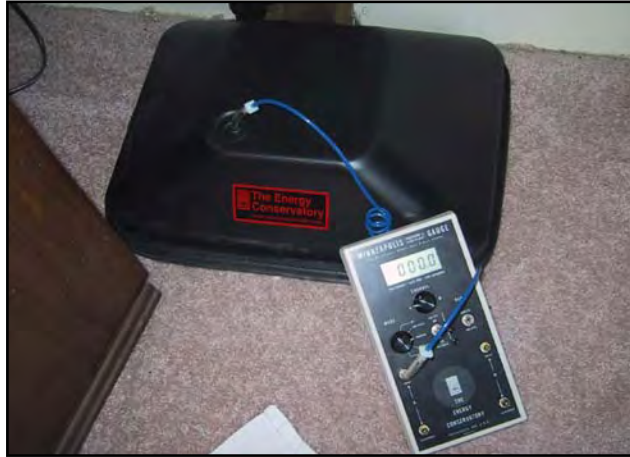
Pressure pan and digital monometer, both from The Energy Conservatory
