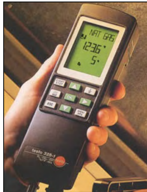
The Testo 325 combustion analyzer measures steady-state efficiency and carbon monoxide emissions
