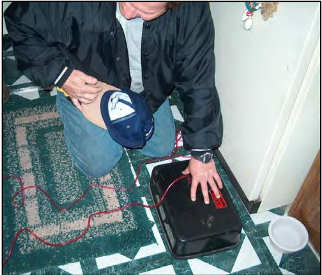
Pressure pan test (operating blower door not pictured)
