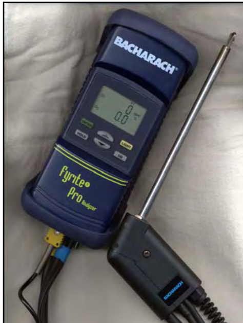
The Bacharach Fyrite Pro combustion analyzer measures steady-state efficiency and carbon monoxide emissions
