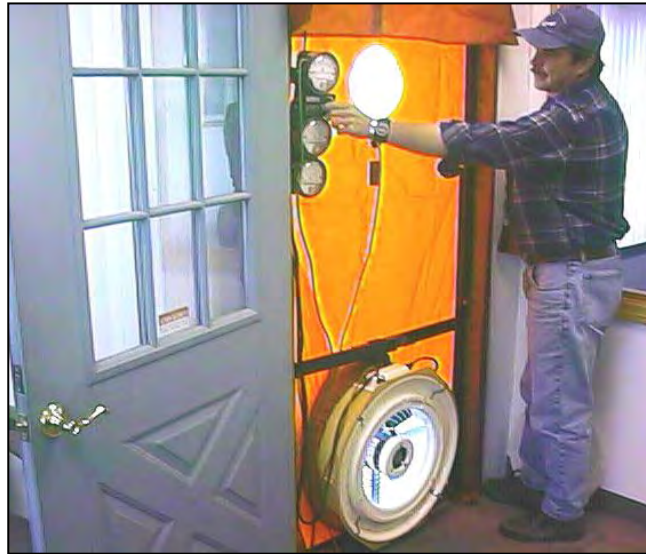
A blower door is needed for the duct blower test to determine leakage to the outdoors
